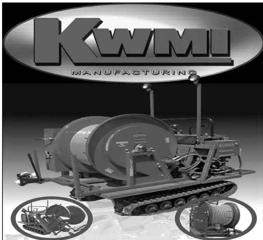
The KWMI Easement Machine is an all-terrain rubber tracked power carrier designed specifically for the pumper-cleaner industry.
