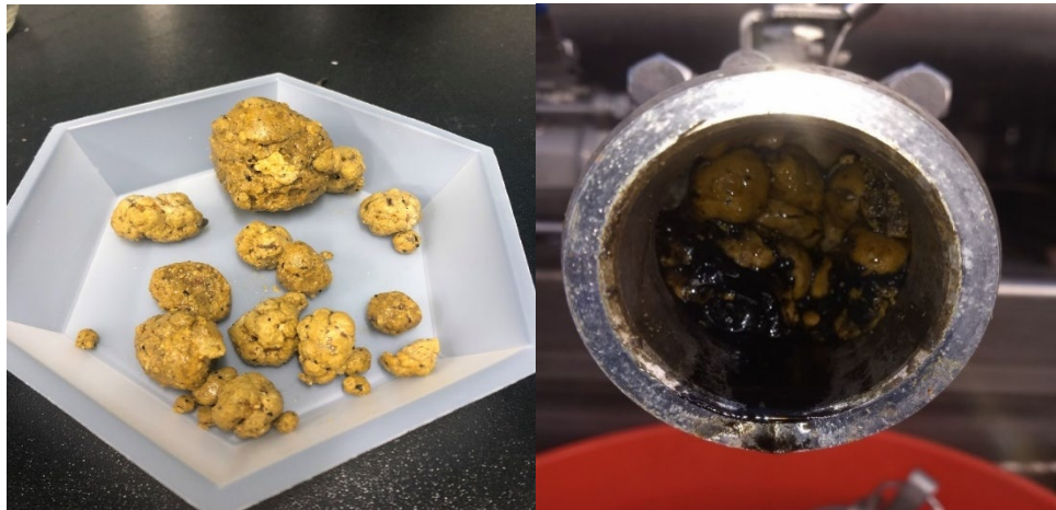
Figure 24: Digester Overflow Blockage and Recovered Clumps
