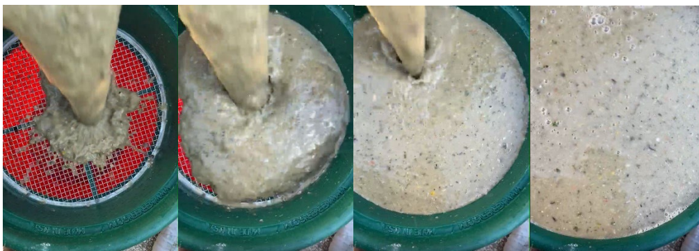
Figure 33: Pre-Thermal Hydrolysis Process Material Screening
