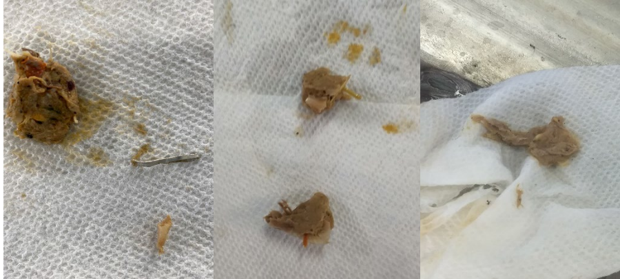
Figure 10: Examples of Food-Based Contaminants Causing Blockages
